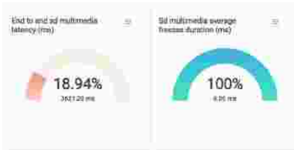
Figure 8: Example of gauge chart visualization components (performance within ‘Acceptable’ range, on the left; and ‘Optimal’ performance case, on the right)
