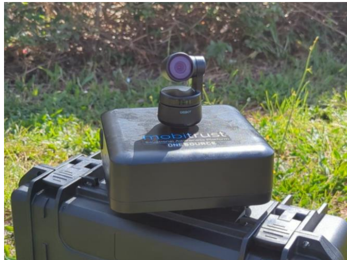
Figure 3: 5G enabled device for sprinklers monitoring and management
