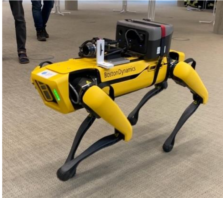
Figure 1 : Boston Dynamics Spot (provided by HHI), carrying the camera Systems, controlled by a Firefighter.
