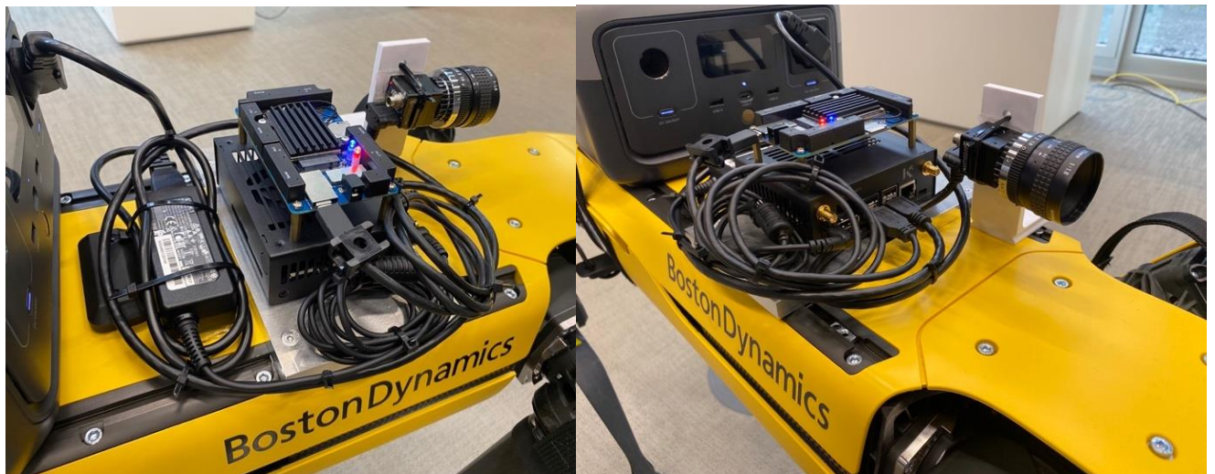
Figure 1 : Boston Dynamics Spot (provided by HHI), carrying the camera Systems, controlled by a Firefighter.
