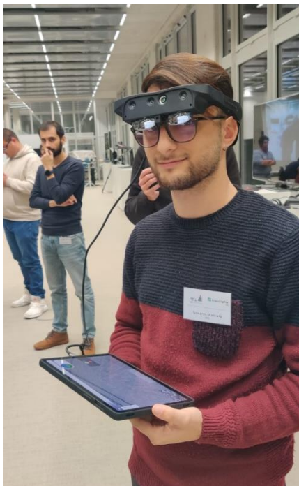
Figure 2: HHI setup with AR visor connected with the Android tablet via USB cable
